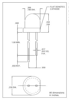
The Ultrabright CMD3X50 Series LED lamp provides exceptional brightness in a very narrow viewing area, in a clear tinted non-diffused package making them excellent for small area backlighting. A pale tint aids in identification. The High Efficiency Red and Yellow lamps are produced with GaAsP/GaP and the High Efficiency Green lamp is produced with GaP/GaP. All feature an 80 mcd minimum luminous intensity.
