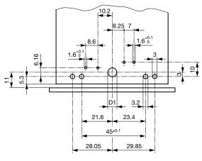
Fixation on PCB or housing from below
