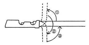
(2) Cut off the insulation barrel at the (a) portion and cut off the wire at the (b) portion. Remove the wire insulation and check the wire conductors for damage.
