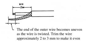
(3) Do not excessively twist the conductors.
