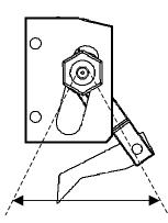
**8-3** When adjusting the pitch always try to feed the terminal on the Insulation bucket as shown in the item 2 below, if this cannot be achieved then using the Conductor bucket is acceptable.
