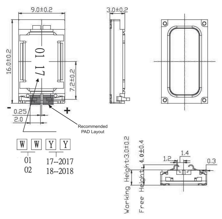
1. Maximum compression force between front frame and back frame & yoke is 5 N.
