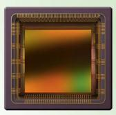
The CMV4000 is a high sensitivity, pipelined global shutter CMOS image sensor with 2048 x 2048 pixel resolution capable of HD format. Pipelining allows exposure during read out. The state-of-the-art pixel
