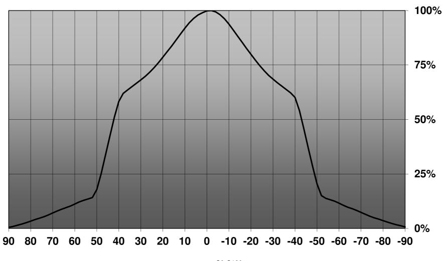
Luminaire: Ledil Oy CN14529\_BROOKE-XW-VERO10\_SIMULATED Lamps: 1 x BRIDGELUX VERO10
