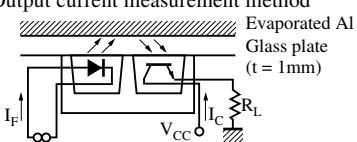
\*<sup>3</sup> Time required for the output current to increase from 10% to 90% of its final value
