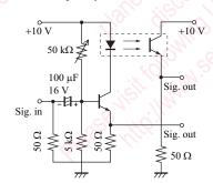
Measurement circuit of frequency characteristics
