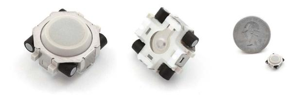
**Description:** This is a tiny trackball akin to those found on a number of Blackberry models (8100, 8300, 8320, 8800, 8830, etc). Each of the four spindles have a tiny circular magnet on each end. Great when paired with very small SMD Hall effect sensors.
