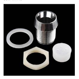
**Description:** These plastic LED holders have a slick chrome finish and make it possible to panel-mount your indicator lights for a clean look. These LED holders accept a 10mm LED and mount into an ½" diameter hole.
