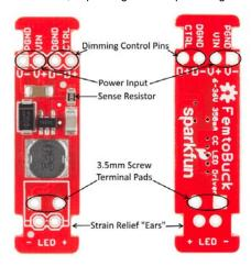
One signal input is provided for dimming control. A ground pin (DGND) is provided to reference against the controlling module for accuracy. Dimming can be done by an analog voltage (20%-100% of max current by varying voltage from .5V-2.5V) or by PWM (so long as PWM minimum voltage is less than .4V and maximum voltage is more than 2.4V) for a full 0-100% range.
