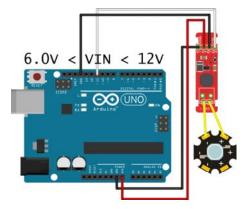
If you have only one or two LEDs, you can connect the FemtoBuck directly to the VIN pin on your Arduino. **You will need to power the board from an external supply**, as the 5V provided by USB isn't high enough to power the FemtoBuck.
