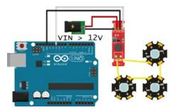
If you have more than a couple of LEDs, you should provide an independent power supply from the Arduino. Multiple LEDs can be connected in series, as shown, and the supply voltage should be at least 2-3V higher than the sum of the forward voltages of the LEDs.
