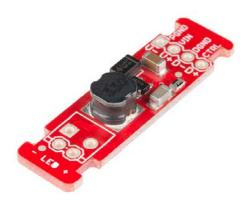
The FemtoBuck is a small-size, single-output constant current LED driver. By default, the FemtoBuck is driven at 350mA. That current can be reduced by either presenting an analog voltage or a PWM signal to the board.
