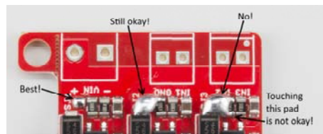
Current Set Resistors
