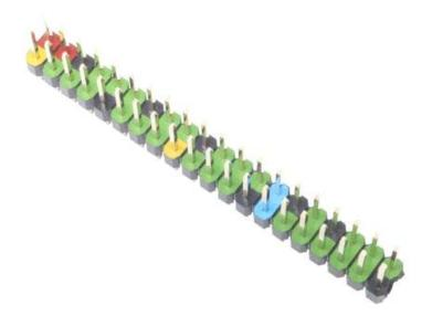
Colour-coded GPIO pins that make locating that ground or power connection you need super simple!
