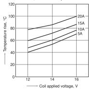
1.-(2) Coil temperature rise Sample: CP1-12V, 6pcs Point measured: Inside the coil Contact carrying current, 5A, 10A, 15A, 20A Resistance method, ambient temperature 85°C 185°F
