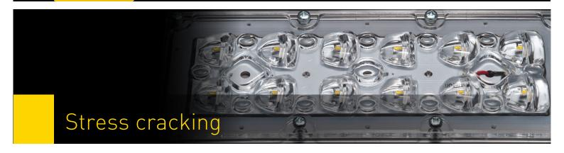
LEDiL products are designed and manufactured to avoid internal stress as much as possible, but this can't be totally avoided. Common optical grade thermoplastics are vulnerable to crack by combination of external or internal stress sources and chemicals.
