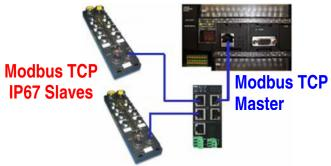
Shown above is a CP1H PLC with a CP1W-MODTCP01-US adapter configured for Master mode. It is communicating to two remote Omron IP67 Modbus TCP slaves. An Omron W4S Ethernet switch is used to connect the various Ethernet devices.
