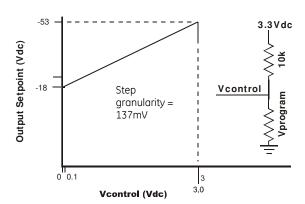
An open circuit on this pin reverts the voltage level back to the original setting of 48V
