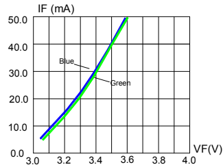
FIG.1 FORWARD CURRENT VS. FORWARD VOLTAGE.
