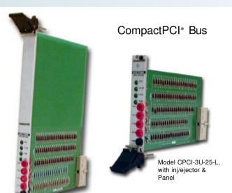
Resistive Load & Voltage Boards for 3U & 6U cPCI Applications
