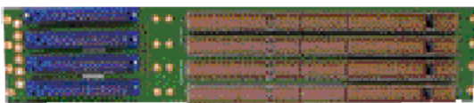
6U cPCI backplane for horizontal card insertion 4 P47 Power Supply Connectors shown
