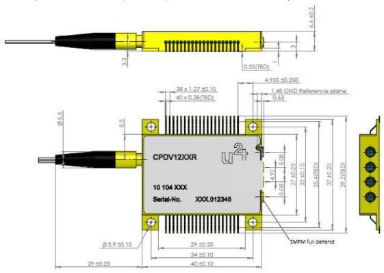
RF interface is realized in GPPO® compatible, male connectors.
