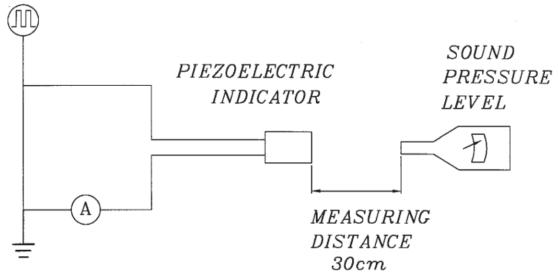
S.P.L. Measuring Circuit Input signal: 12 V p-p, 3.0 kHz, square wave Mic: RION S.P.L. meter UC30 or equivalent
