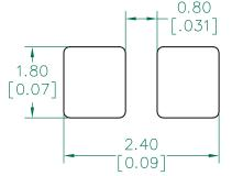
(For wave soldering, add 0.763 [0.030] to this dimension)
