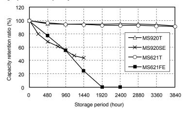
MS-T series's capacity retention ratio after High temperature storage were greatly improved.
