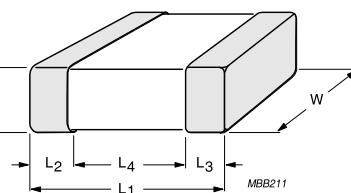
Fig. 2 Surface mounted multilayer ceramic capacitor dimension
