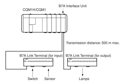
**Note** The maximum transmission distance depends on the transmission delay time and the power supply wiring.
