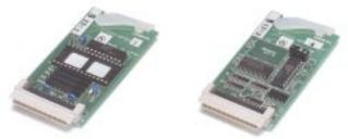
Choose either the EEPROM or the EPROM Memory Cassette to enhance the CQM1's memory. They will prevent the CQM1's Program Memory and DM from being lost during power interruption. The program and data in DM can be transferred between the CPU unit's RAM and the Memory Cassette. Data cannot be written to EPROM from the CPU unit.
