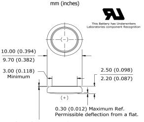
0.03 (0.001) Minimum Ref. (Applies to top edge of gasket or edge of crimp, whichever is higher.) Classification: Chemical System: Designation: Nominal Voltage: Typical Capacity:
