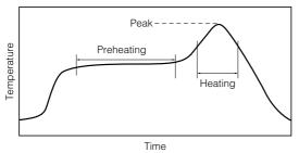
For soldering (Example : Sn/Pb)
