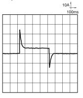
9-(2). Electrical life test (Motor lock) Sample: CR2-12V, 3pcs Brake current: 22A, power window motor actual load (lock condition) Tested voltage: 14V DC Switching frequency: (ON:OFF = 0.5s:9.5s) Ambient temperature: Room temperature
