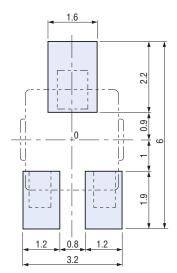
Note 1) The zero point is the center of mounting.
