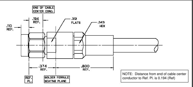
3.1 Insert cable/contact sub-assembly into connector until seated and tighten clamp nut to 25-35 in-lbs.
