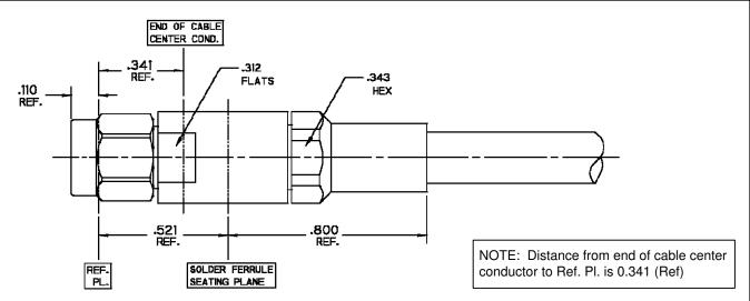
3.1 Insert cable/contact sub-assembly into connector until seated and tighten clamp nut to 25-35 in-lbs.
