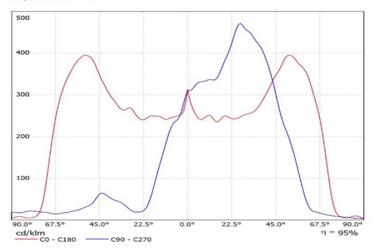
Luminaire: Ledil Oy CS15389\_STRADA-2X2MX-T2-S\_(XHP70)\_SIMULATED Lamps: 1 x Cree XHP70 - 1.00 W
