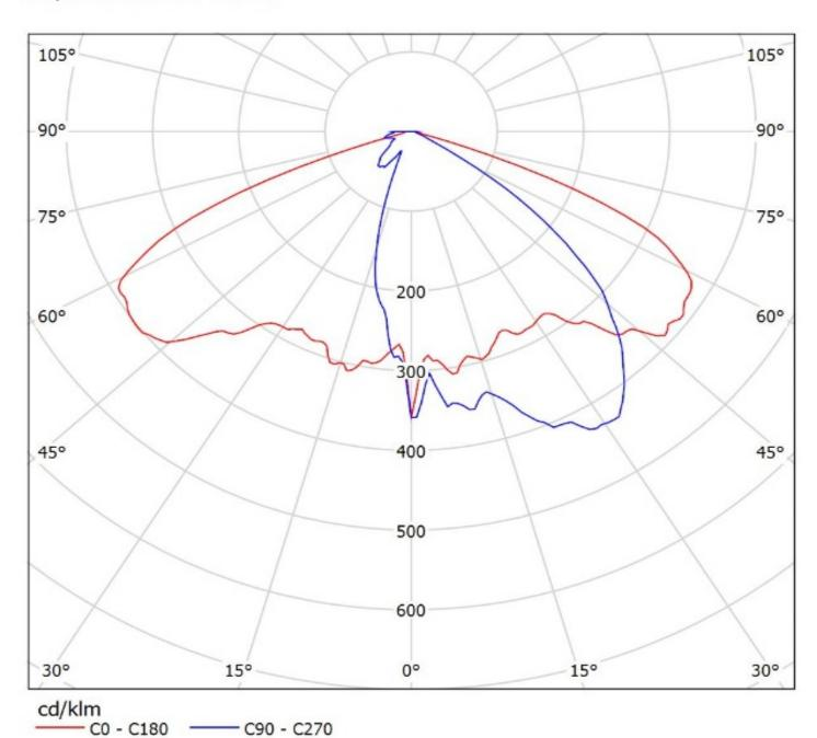
Luminaire: Ledil Oy CS15389\_STRADA-2X2MX-T2-S\_LUXEON\_MX\_SIMULATED Lamps: 1 x LUXEON MX
