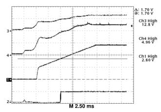
Trace 3 – 12 V Input (V<sub>CC1</sub>) and (V<sub>CC2</sub>) (10 V/div.)
