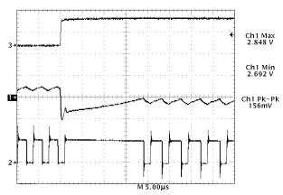
Trace 1- Regulator Output Voltage (100 mV/div.)
