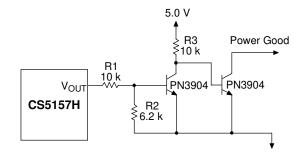
Figure 17. Implementing Power Good with the CS5157H
