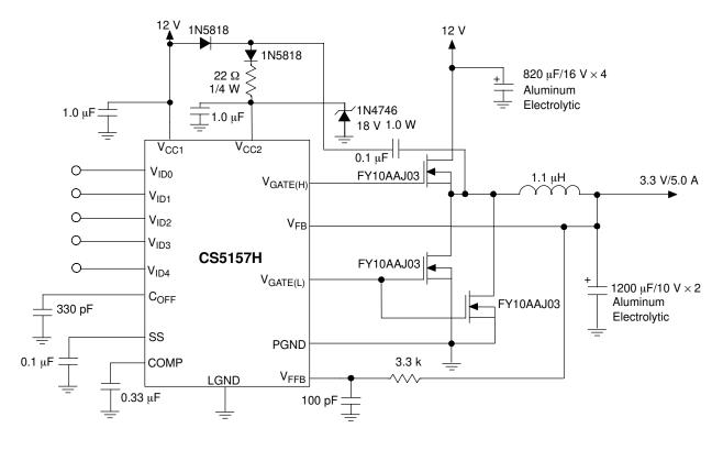
Figure 26. Additional Application Diagram, 12 V to 3.3 V/5.0 A Converter with Remote Sense
