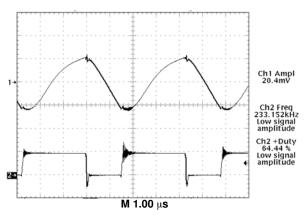
Trace 1 – Regulator Output Voltage (10 mV/div.)
