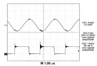
Trace 1– Regulator Output Voltage (10 mV/div.)
