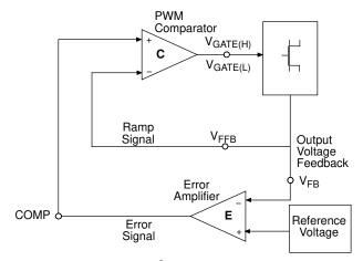
Figure 3. V<sup>2</sup> Control Diagram
