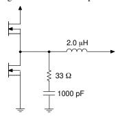
Figure 20. Filter Components
