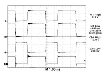
$$\begin{split} &\text{Trace 3} = V_{GATE(H)} \; (\text{10 V/div.}) \\ &\text{Math 1} = V_{GATE(H)} - 5.0 \; V_{IN} \\ &\text{Trace 4} = V_{GATE(L)} \; (\text{10 V/div.}) \end{split}$$
