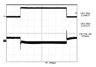
Trace 1- Regulator Output Voltage (100 mV/div.)
