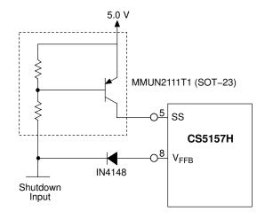
Figure 16. Implementing Shutdown with the CS5157H
