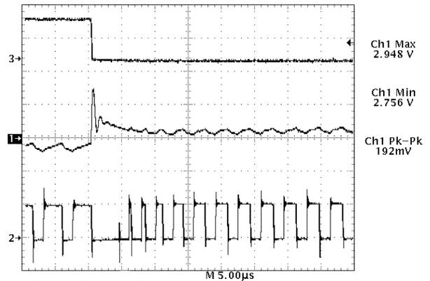
Trace 1– Regulator Output Voltage (100 mV/div.)
