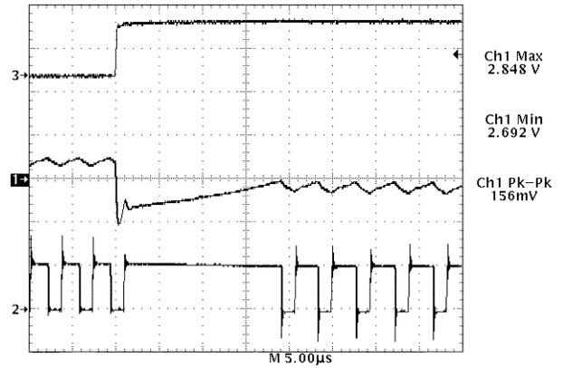
Trace 1– Regulator Output Voltage (100 mV/div.)
