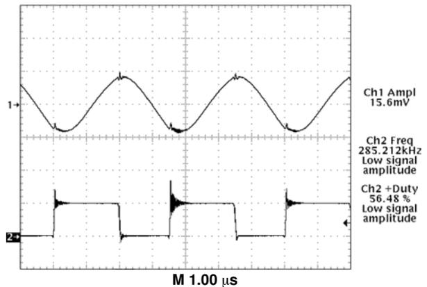
Trace 1– Regulator Output Voltage (10 mV/div.)
