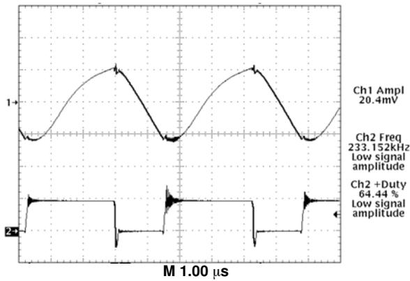
Trace 1– Regulator Output Voltage (10 mV/div.)
