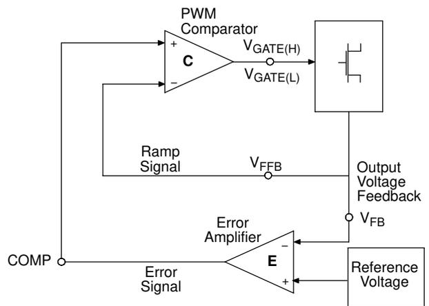
Figure 3. V<sup>2</sup> Control Diagram
