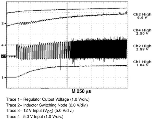
**Figure 10. Demonstration Board Startup in Response to Increasing 12 V and 5.0 V Input Voltages. Extended Off Time is Followed by Normal Off Time Operation when Output Voltage Achieves Regulation to the Error Amplifier Output.**
