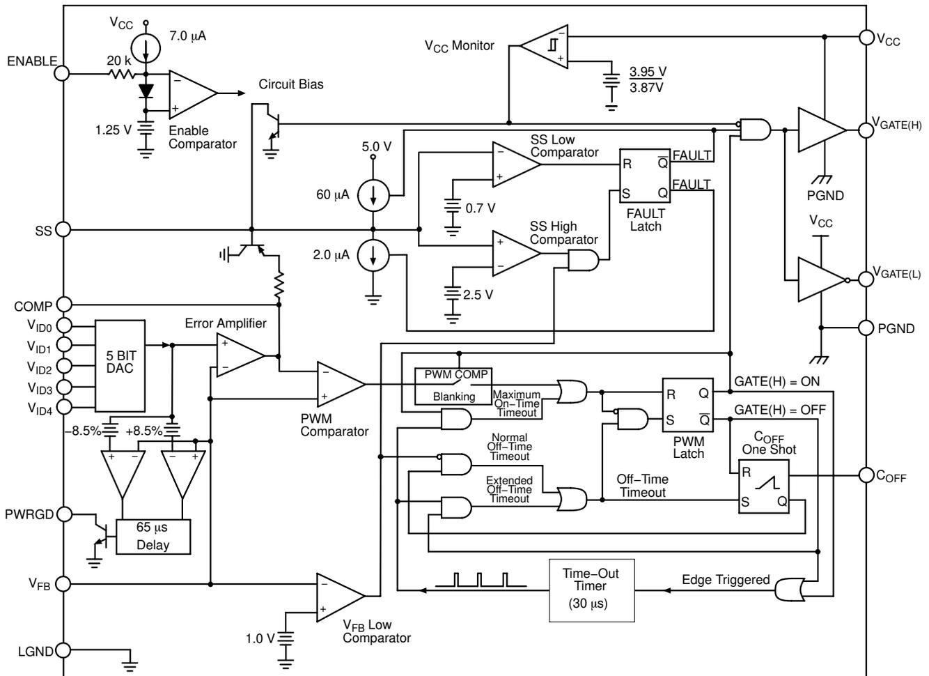
Figure 2. Block Diagram
