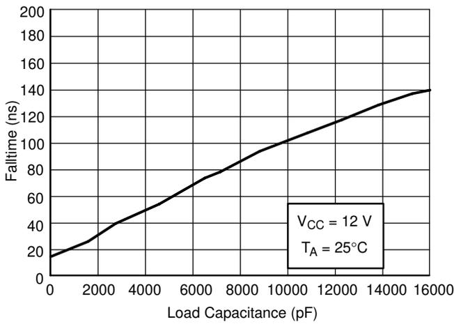
Figure 5. GATE(H) & GATE(L) Falltime vs. Load Capacitance
