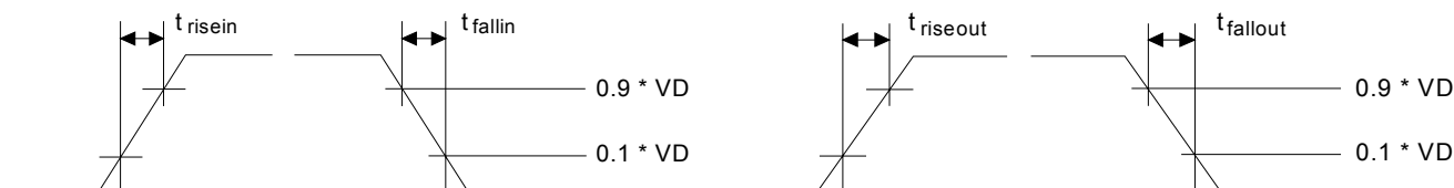
Figure 1. Rise and Fall Times
