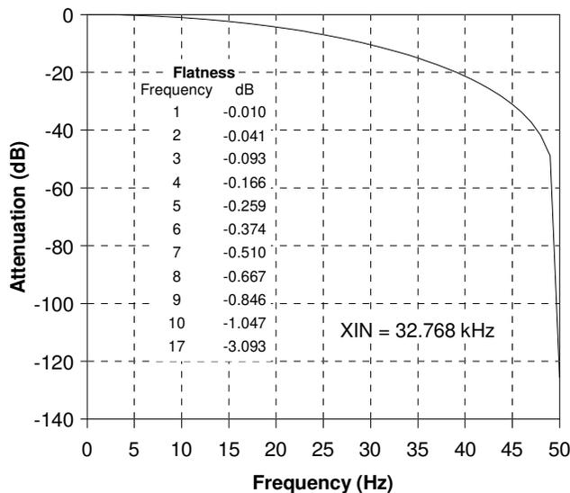
**Figure 7. Filter Magnitude Plot to 50 Hz**
