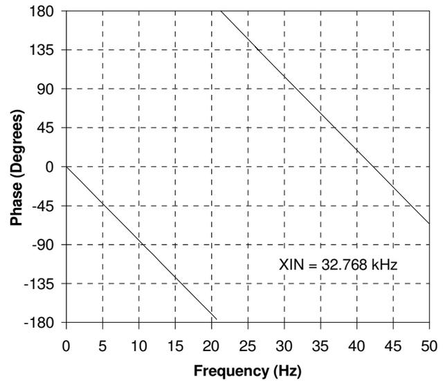
**Figure 8. Filter Phase Plot to 50 Hz**
