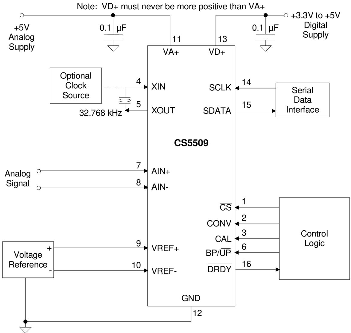
Figure 9b. System Connection Diagram Using Split Supplies
