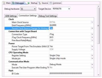
20. If using an external power supply, ensure that the "Power Target from the Emulator" option is set to No. (See the RSKRX63T User Manual for power supply options and board settings.) The board is configured by default to run from emulator power.
