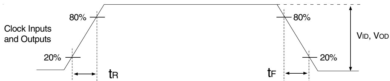
Figure 8. Input and Output Slew Rates
