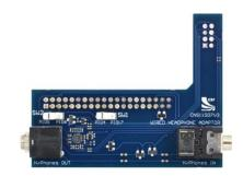
This board allows the developer to design a product which includes the ability to operate in a wired mode (non-Bluetooth) with the BlueCore® CSR8670 WLCSP powered off.
