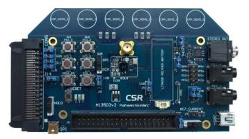
This board features the latest CSR BlueCore® CSR8675 WLCSP Bluetooth audio solution. It interfaces with microphones and has flexible LED and push-button assignments. Battery current measurements can be performed, and a PIO header allows for connection of further application hardware, such as displays.
