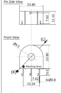
All dimensions are in mm Linear dimensional tolerance ±0.2mm
