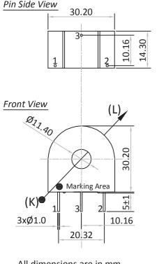
All dimensions are in mm Linear dimensional tolerance ±0.2mm
