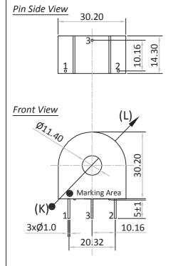
All dimensions are in mm Linear dimensional tolerance ±0.2mm
