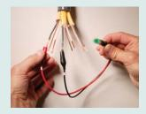
GREEN LED means wiring is properly identified.
