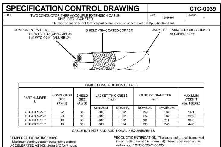
The "\*\*" in the product identification shall be replaced by the AWG size, color sequence of components, and jacket color. For example, if AWG size is 16 and color code is per MIL-STD-687, the "\*\*" should be replaced with "16-9/5-9".
