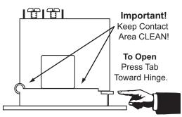
Run wire to be monitored through opening in the sensor. The CTL Series transducers work in the same environment as motors, contactors, heaters, pullboxes, and other electrical enclosures. They can be mounted in any position or hung directly on wires with a wire tie. Just leave at least one inch (25.4 mm) distance between sensor and other magnetic devices.
