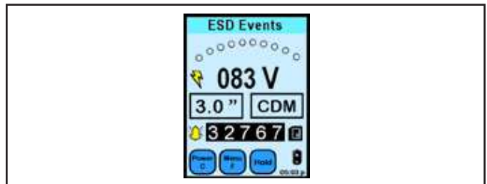
Figure 21. ESD Event voltage display
